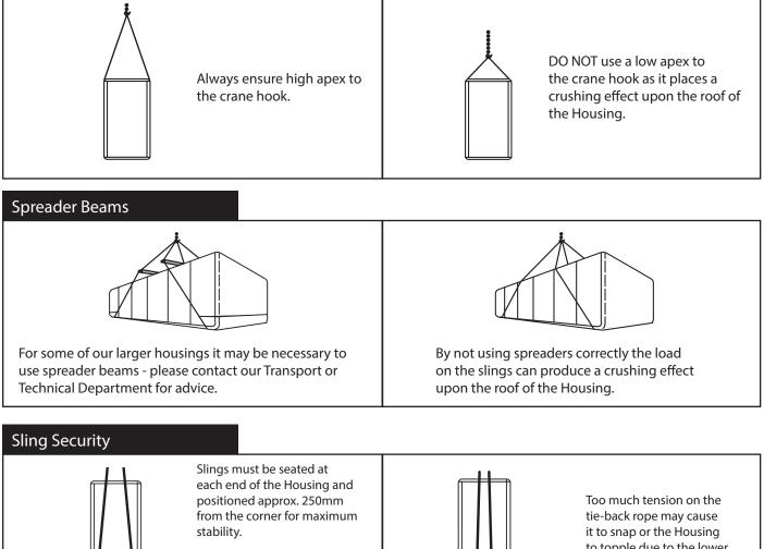
Always tension the slings before tying back and place tie-back ropes at low level to prevent the slings from slipping inwards as indicated on page 12.
